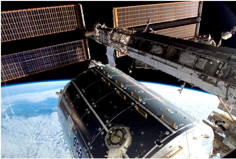
Figure 14: Whipple Shields on ESA's Columbus module of the ISS (cylinder shape). Credits: ESA.
