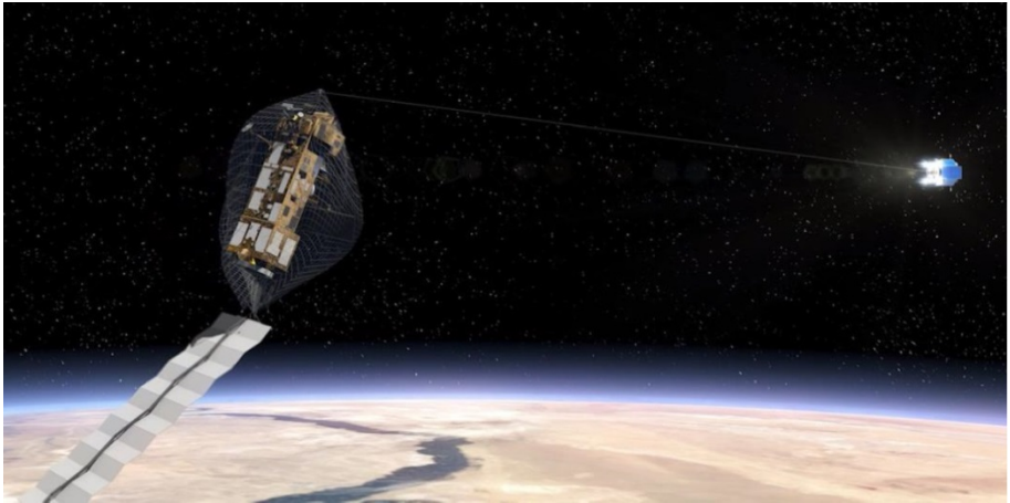
Figure 56: e.deorbit capturing the target with a net. Credits: Airbus Defence and Space [RD15].
