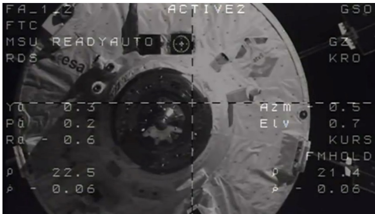
Figure 47: The Automated Transfer Vehicle 5 (ATV-5) docks to the ISS using very similar sensors required to capture debris, such as a LIDAR. Credits: ESA.
