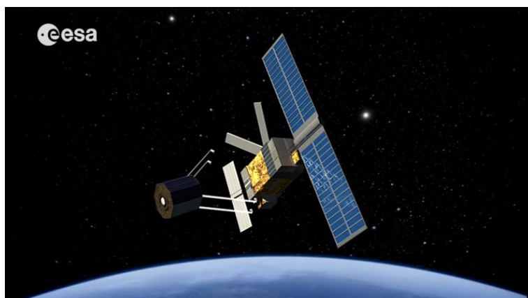
Figure 39: Example of a chaser using a clamping mechanism to capture a target. Credits: ESA.
